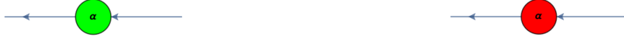
Figure 19: Z- and X-spiders with input arities of 1 and output arities of 1, corresponding to the expressions Z[z_1, 1, 1, \alpha] \otimes (W[i_1, z_1] \otimes W[z_1, o_1]) and X[x_1, 1, 1, \alpha] \otimes (W[i_1, x_1] \otimes W[x_1, o_1]) , respectively, are interpreted as unitary maps.
