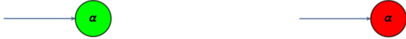
Figure 22: Z- and X-spiders with input arities of 1 and output arities of 0, corresponding to the expressions Z[z_1, 1, 0, \alpha] \otimes W[i_1, z_1] and X[x_1, 1, 0, \alpha] \otimes W[i_1, x_1] , respectively, are interpreted as projections.
