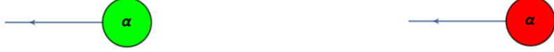
Figure 18: Z- and X-spiders with input arities of 0 and output arities of 1, corresponding to the expressions Z[z_1, 0, 1, \alpha] \otimes W[z_1, o_1] and X[x_1, 0, 1, \alpha] \otimes W[x_1, o_1] , respectively, are interpreted as pure states.
