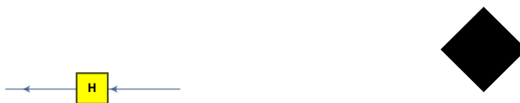
Figure 23: The Hadamard and black diamond spiders, corresponding to the expressions H[h_1, \cdot] \otimes (W[i_1, h_1] \otimes W[h_1, o_1]) and B[d_1] , are interpreted as Hadamard transformations and overall (multiplicative) scalar factors, respectively.
